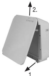
2. Remove the housing cover as shown (magnetic fastening). Firstly detach the magnetic fastening at the bottom, and then at the top.
